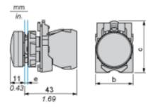
**e:** clamping thickness: 1 to 6 mm / 0.04 to 0.24 in. **b:** 30 mm / 1.18 in.
